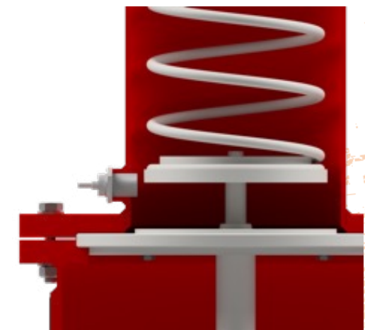
Fig. 4: Sectional drawing of an in line pressure or vacuum valve with proximity switch
